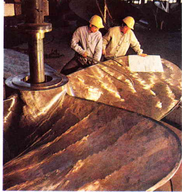
Propeller being examined for quality.
